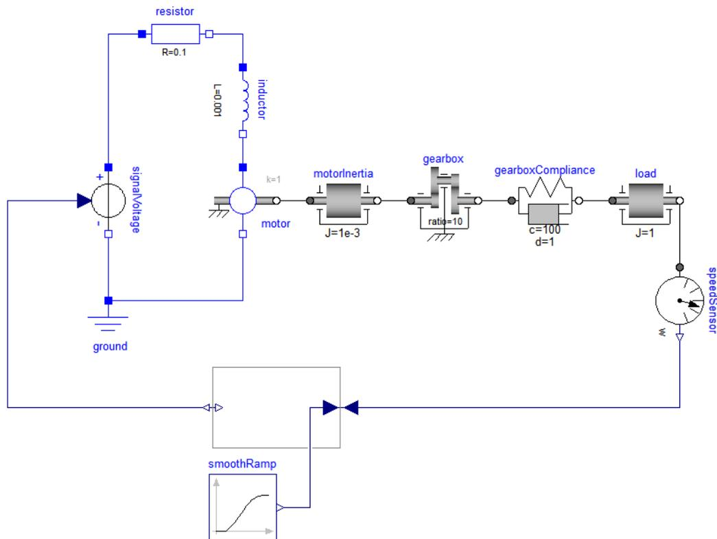
The physical model is reused without modification, all we have done is disconnect the existing control system model and add two new components to the model to actuate it in a different way.
