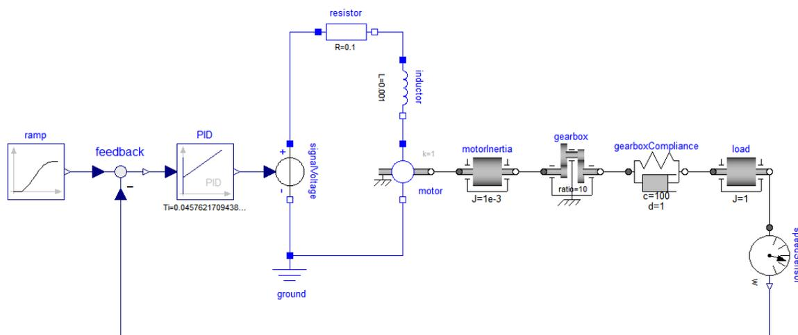
Suppose we want to approach the problem from a different perspective and we want to explore how the motor power requirement is affected by changes in the compliance of the mechanical
