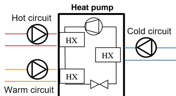
Figure 2: Schematic of the heat pump and liquid fluid circuits.
