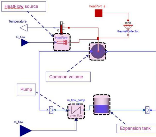
Figure 3: Schematic of the liquid fluid circuit model.
