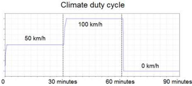
Figure 4: Duty cycle for system testing.
