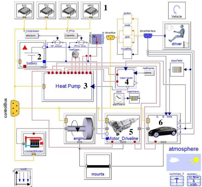
Figure 1: Diagram of overall vehicle model architecture. 1 - Controllers for transmission, electric drives and heat pump system, 2 – BEV battery, 3 – Heat pump model including fluid circuits, 4 - Cabin model, 5 - Transmission model, 6 – Chassis and brakes model.
