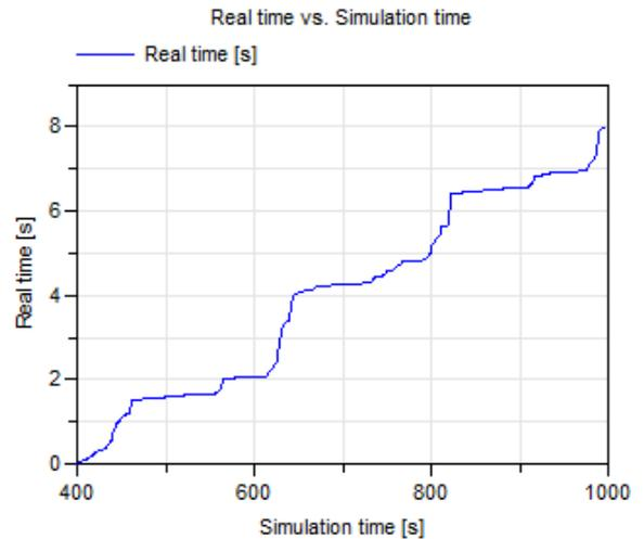
**Figure 14:** Model performance using Radau IIa variable stiff solver for stiff systems showing Real time (vertical axis) vs. simulation time (horizontal axis).
