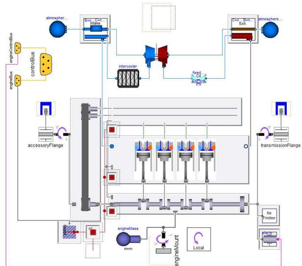
**Figure 5:** Mean Value engine model with replaceable mechanical and fluidic subsystems.
