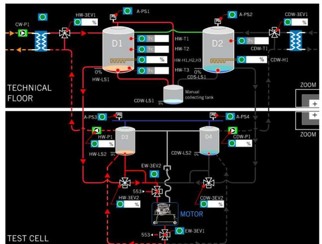
**Figure 2:** Example of an engine thermal shock rig showing the main components and routing, including the equipment split between the technical floor and the test cell.
