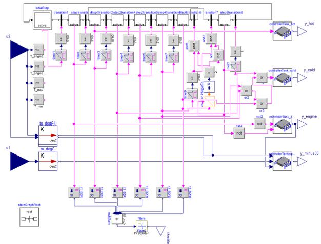
**Figure 10:** StateGraph controllers for the 3-way valves.
