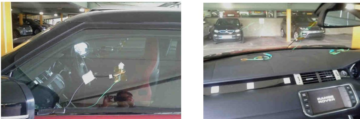
**Figure 1.0: Thermocouple locations on glazing and defrost vents**
