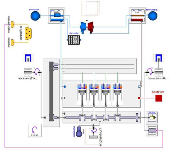
Figure 5: In-line 4 cylinder direct injection gasoline turbocharged mean value engine model diagram
