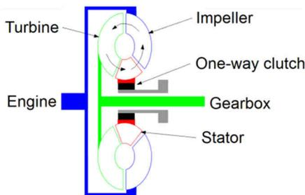
Figure 2: Torque converter mechanical schematic with fluid flow arrows in the driven condition
