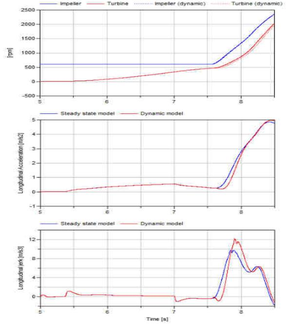
Figure 7: Impeller and turbine speed (top), vehicle acceleration and Jerk (bottom) comparison
