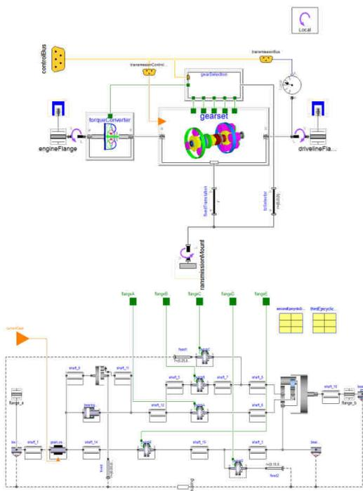
Figure 3: Model Diagram of automatic transmission (top) and gearset (bottom)
