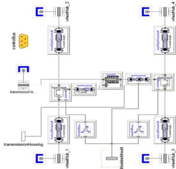
Figure 4: Template for four wheel drive
