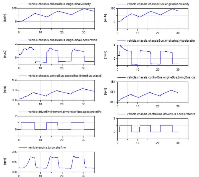
Figure 6: Vehicle simulation results for a 1.8l I4 DI SI Turbo (left) and 2.7l V6 DI SI NA (right). x-axis: time(s)
