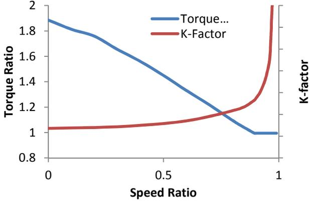
Figure 1: Steady state torque converter curves
