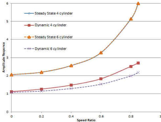
Figure 8: Amplitude response for both engines with steady state and dynamic torque converter models.
