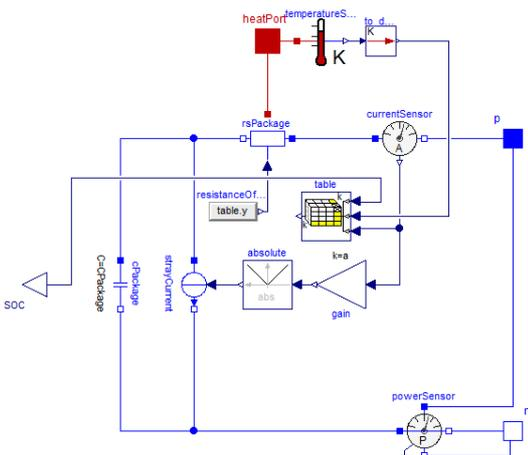
Figure 4: ERS equivalent circuit battery model
