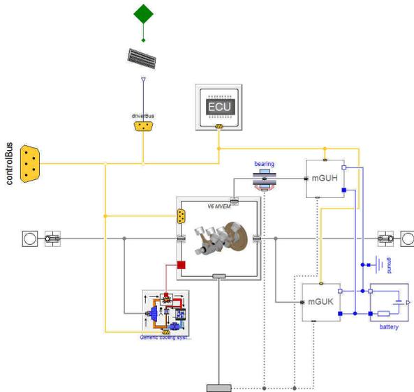
Figure 3: Engine model including ERS, ECU and cooling system
