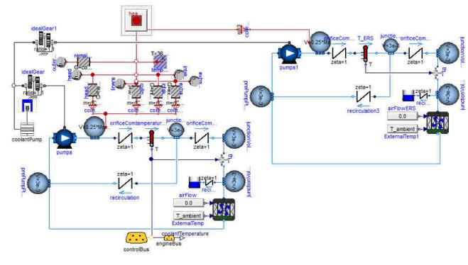
Figure 5: Engine Cooling System modelled as a 1D thermofluid system. Engine cooling on left and ERS cooling loop on right.
