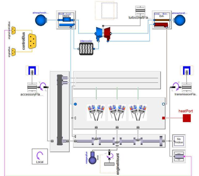
Figure 2: V6 turbocharged engine model
